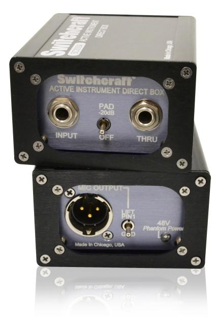
A 48V phantom powered instrument direct box designed to quietly preserve the tone of the world's finest musical instruments. The SC800A is ideal for converting the unbalanced outputs of passive musical instruments such as acoustic guitar and bass to balanced, mic level signals that can be connected to audio consoles and mic preamps. Precision engineered active circuitry provides extended reach and superior audio fidelity for professional audio engineers and musicians
